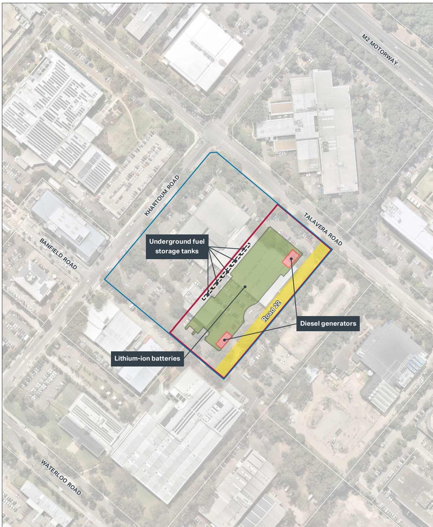
Figure 15-1 Location of back-up generators, diesel fuel storage tanks and lithium-ion batteries
